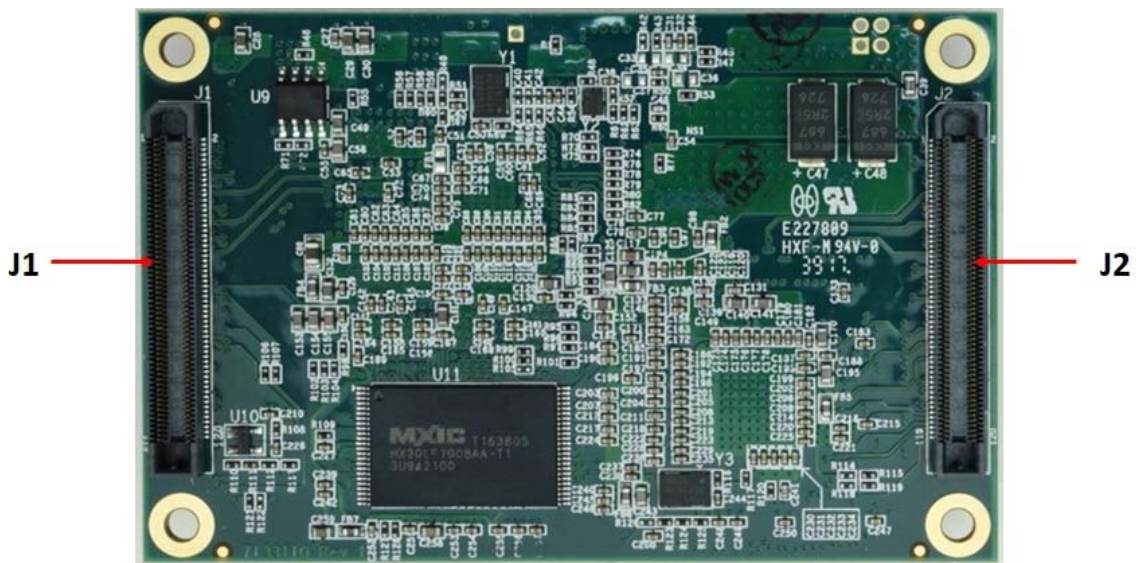
Figure 6-2: Bottom View of J-Pin Connectors on EPSM-10GX
